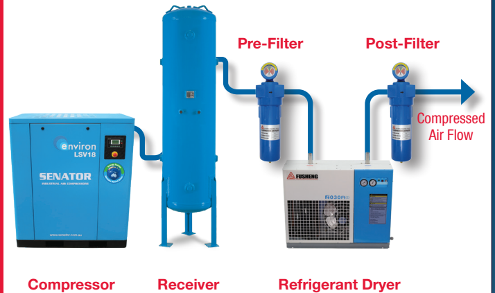
Typical Industrial Compressed Air System
