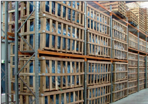
Standard Pallet Racking Storage ≤ 1,240 Litres
