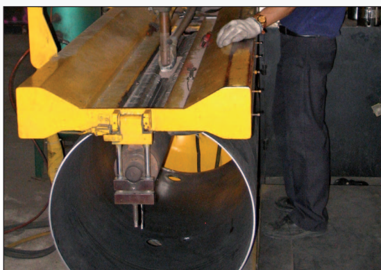
Longitudinal Joint Welding
